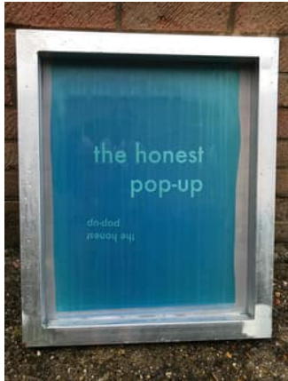
THE SCREEN, EXPOSED Hickman Design · Washing out exposed screen printing emulsion 03 · 2019 · Hickman Design, CC BY-SA 4.0, via Wikimedia Commons
